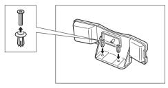
2 Insert the plugs with the handset cradle in the holes on the machine.
